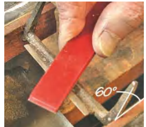
▲ Pic.10 A diamond hone can do the job of forming the 30° sharpening angle
